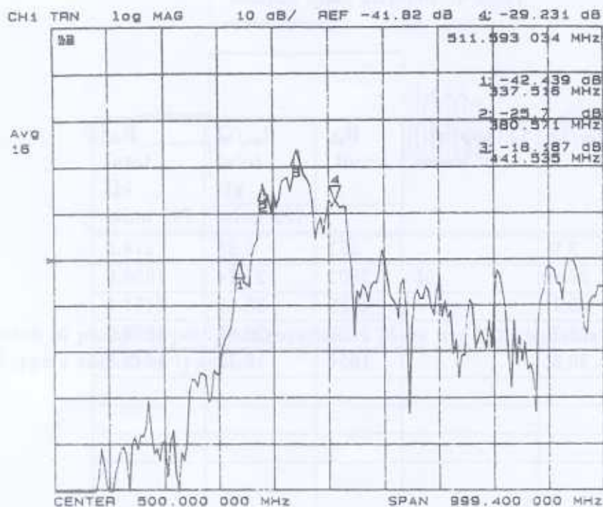
Figure 3: Laboratory measurement of the resonant frequencies of the MSE. With the excitation used both longitudinal and transverse resonances may be seen.
